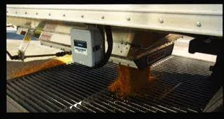
Timpte hopper tubs are made of formed aluminum sheets. Design allows product to flow freely. Rubber flaps eliminate any potential water intrusion. All Timpte trailers are standard with liquid filled air scale gauge and dump valve in a weatherproof box.
