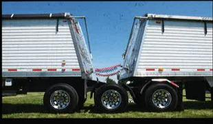
Timpte "B Train" is standard with a 15 degree slope on the rear of the lead and the front of the pup. The tri-axle sub frame is designed to be clean, light weight, but not light duty. The sub frame is designed to handle the rigors of the Canadian weather and is coated with "Black Armor" to protect from corrosive elements.
