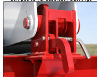
Secure Manual Latch System with Composite (Greaseless) Bushings
